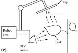
Fig. 1. Autonomous pest control robot (Cabbot). (a) Cabbot in operation, (b) sampling device, (c) schematic diagram of sticky trap with angle ( $\theta$ ) for collecting whiteflies.
