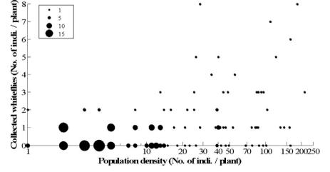
Fig. 5. Frequencies of sampling in different number of whiteflies by the Cabbot across different level of total population size in logarithmic scale. Size of circles indicates frequency of samples with the collected number of whiteflies per plant.
