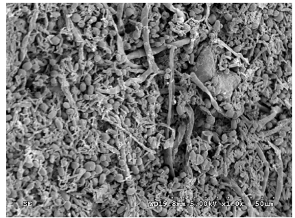
图 7 沸石表面电镜照片 (×1 000) Fig. 7 Electron microscope of zeolite surface with microorganism (×1 000)
