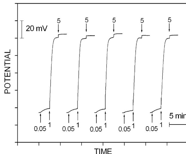
Fig. 2. Electrode regenerability of the proposed technique. Before each measurement, the electrode was thoroughly rinsed and allowed to be activated in 0.12 M  $\text{Na}^+$  for 20 min; after each measurement a new round was performed without the reconditioning step. Protamine concentrations ( $\mu\text{g}/\text{mL}$ ) are indicated on the traces.
