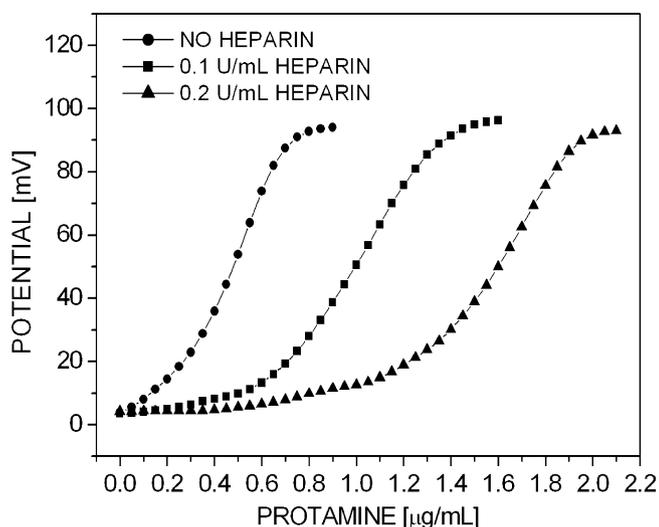
Fig. 3. Potential curves for the titration of heparin in 0.12 M NaCl with protamine using the same proposed PrSE. The titration interval was 30 s.
