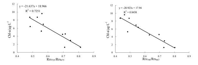
Fig. 6. Relationship between the Chl-a Concentration and the band ratio.
