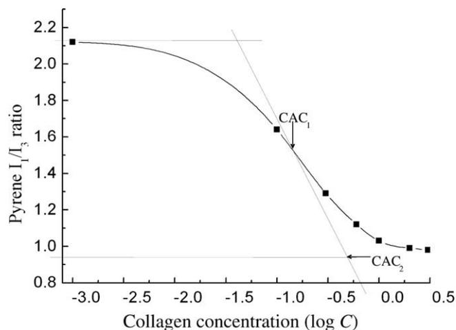
Fig. 2. Plots of pyrene  $I_1/I_3$  ratio versus the logarithm of different concentrations of acid-soluble collagen from walleye pollock skin in Na-phosphate buffer at pH 7.2 after incubation for 72 h at 37  $^{\circ}\text{C}$ .
