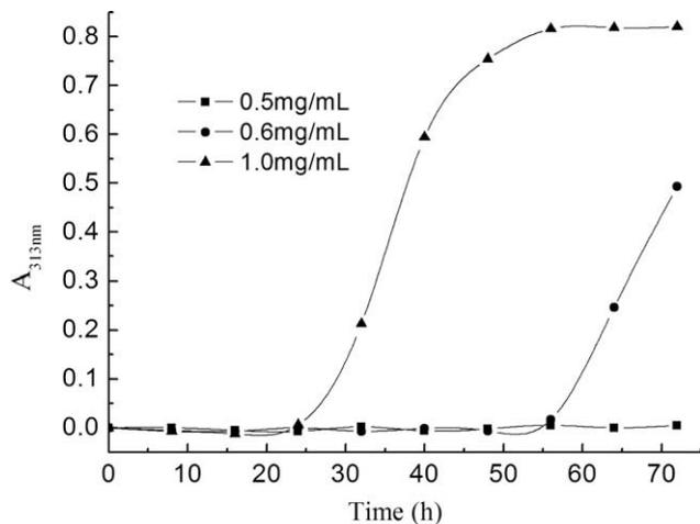
**Fig. 3.** Aggregation kinetics of collagen from walleye pollock skin at different concentrations in Na-phosphate buffer at pH 7.2 and 37 °C (closed square, 0.5 mg/ml; closed circle, 0.6 mg/ml; closed triangle, 1.0 mg/ml).
