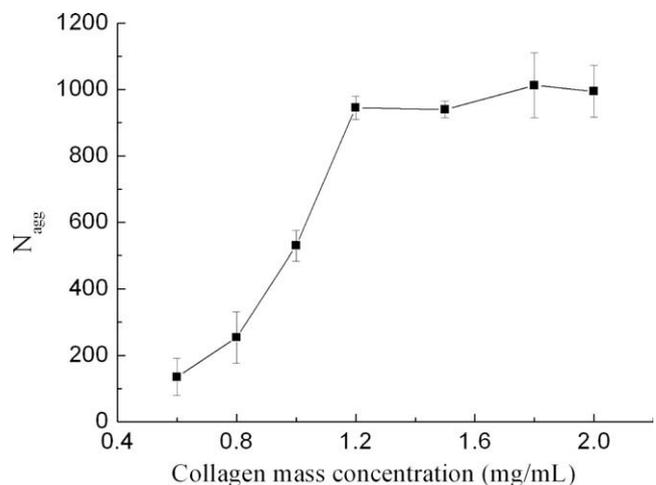
**Fig. 5.** Aggregation numbers of acid-soluble collagen from walleye pollock skin at different concentrations in Na-phosphate buffer at pH 7.2 and 37 °C.
