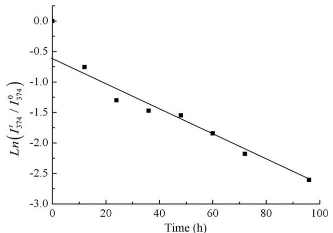
**Fig. 4.** Plots of the natural logarithm of pyrene  $I_{374}^t/I_{374}^0$  versus time in the acid-soluble collagen (0.6 mg/ml)/Na-phosphate buffer system at 37 °C.
