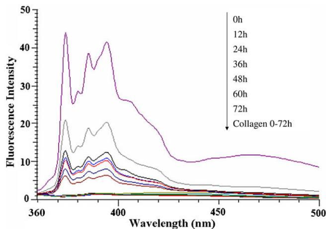
Fig. 1. Fluorescence spectra of pyrene (2  $\mu\text{M}$ ) and acid-soluble collagen from walleye pollock skin (0.6 mg/ml) in the collagen/Na-phosphate buffer system at 37  $^{\circ}\text{C}$ .
