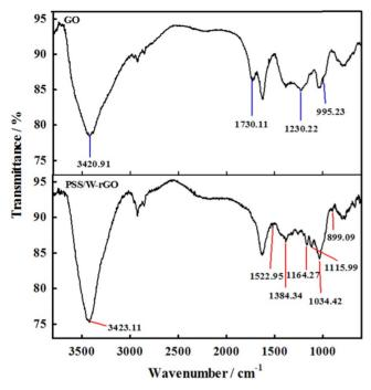
Figure 2. FT-IR spectra of GO, PSS/W-rGO.
