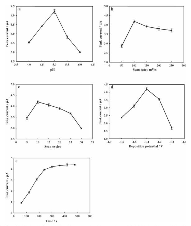
Figure 6. Effects of the pH values (a) of acetate buffer solution, scan rate (b) and the scan cycles (c) of 0.2 mM PSS, deposition potential (d) and the deposition time (e) on the DPV peak current for 230 nM Zn(II) in 0.1 M acetate buffer solution at the PSS/W-rGO/GCE. n = 3.
