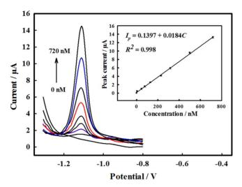
**Figure 7.** DPV voltammograms of the PSS/W-rGO/GCE in 0.1 M acetate buffer (pH 5.0) containing different Zn(II) concentrations (5 to 720 nM). Parameters: amplitude of 0.05 V, a pulse width of 0.2 s, pulse period of 0.5 s, and an equilibrium time period of 2 s. Left: The calibration curve for Zn(II) detection (n = 3).
