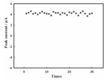
**Figure 8.** Repeatability of the modified-electrode (PSS/W-rGO/GCE) for 30 times measurements in 0.1 M acetate buffer solution (pH 5.0) containing 230 nM Zn(II).
