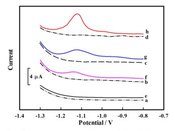
**Figure 5.** DPV response curves in 0.1 M acetate buffer (pH 5.0) without (a)–(d) and with (e)–(h) 230 nM Zn(II) at bare GCE (a), (e), W-rGO/GCE (b), (f), PSS/GCE (c), (g), and PSS/W-rGO/GCE (d), (h). Parameters: amplitude of 0.05 V, pulse width of 0.2 s, pulse period of 0.5 s, and an equilibrium time period of 2 s.
