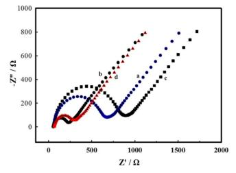
**Figure 4.** Nyquist plots of bare GCE (a), W-rGO/GCE (b), PSS/GCE (c), and PSS/W-rGO/GCE (d) in 0.1 M KCl solutions containing 5 mM  $Fe(CN)_6^{3-/4-}$ .
