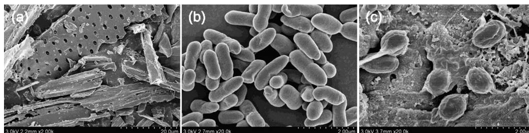
Fig. 1. Scanning electron micrographs of biochar (a), NT-2 strain (b), and NT-2 loaded biochar (c).
