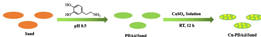
Scheme 1. The fabrication process of Cu-PDA@Sand catalyst through dopamine chemistry including the polydopamine coating and the chelation of Cu ions on the sand support.
