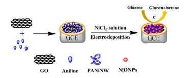
A non-enzymatic glucose biosensor was developed by one-step electrodeposition fabrication of nickel oxide nanoparticles/polyaniline nanowire hybrids on graphene oxide/glassy carbon electrode.
