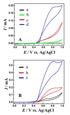
**Fig. 3** (A) CV of GO/GCE (a), PANI/GO/GCE (b), NiONS/GO/GCE (b), and NiONPs/PANiNW/GO/GCE (c) in 0.1 M NaOH containing 2 mM glucose at a scan rate of 100 mV s<sup>-1</sup>. (B) CV of NiONPs/PANiNW/GO/GCE in 0.1 M NaOH containing glucose of varying concentrations at a scan rate of 100 mV s<sup>-1</sup>: (a) 1 mM; (b) 2 mM; (c) 5 mM.
