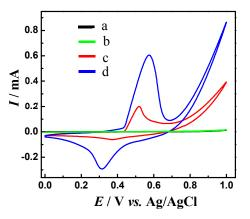
Fig. 2 CVs of GO/GCE (a), PANI/GO/GCE (b), NiONS/GO/GCE (c), and NiONPs/PANiNW/GO/GCE (d) in 0.1 M NaOH at a scan rate of 100 mV s $^{-1}$ .
