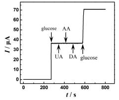
Fig. 5 Amperometric responses of NiONPs/PANiNW/GO/GCE to successive additions of 0.1 mM glucose, 0.1 mM UA, 0.1 mM AA, 0.1 mM DA and then 0.1 mM glucose at +0.6 V in 0.1 M NaOH.
