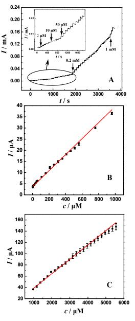
**Fig. 4** (A) Chronoamperometric responses of NiONPs/PANiNW/GO/GCE to successive additions of glucose to 0.1 M NaOH at + 0.6 V. Inset: amplified calibration plot corresponding to the lower concentration range. Calibration plots between the current and glucose concentration in the range from 2  $\mu$ M to 960  $\mu$ M (B), and from 960  $\mu$ M to 5.560 mM (C), respectively.
