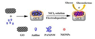
**Scheme 1** Schematic illustration of the enhanced electrochemical detection strategy for glucose based on NiONPs/PANiNW/GO modified on the GCE.
