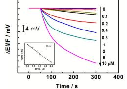
Fig. 4 Typical potential responses of the solid-contact electrode based on 55 MIP to neutral BPS in the concentration range of 0.1 to 10 µM. The inset shows the calibration curve for neutral BPS detection. Other conditions are as given in Fig. 3. Error bars represent one standard deviation for three measurements.
