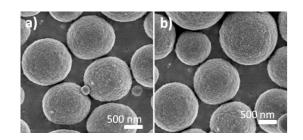
Fig. 1 SEM images of the obtained (a) MIP and (b) NIP beads.
