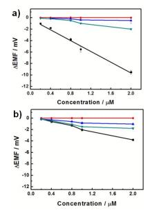
**Fig. 5** Potentiometric selectivity of the MIP (a) and NIP (b) membrane-based 5 sensors towards neutral phenols: (**1**), BPS; (**V**), 2-phenylpheno; (**A**), 4,4 - dihydroxybiphenyll; (**•**), phenol. Other conditions are as given in Fig. 3. Error bars represent one standard deviation for three measurements.
