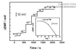
deprotonated BPS. Experimental conditions: membrane composition (in wt%), 1.5 % TDMAC, 2.0 % ETH 500, 35.9 % PVC, 54.6 % DOP and 6.0 % MIP; detection background, 30 mM NaHCO<sub>3</sub>/Na<sub>2</sub>CO<sub>3</sub> buffer of pH 10.2; conditioning solution, 10<sup>-4</sup> M BPS in 30 mM NaHCO<sub>3</sub>/Na<sub>2</sub>CO<sub>3</sub> buffer of pH 40 10.2. The inset shows calibration curve for detection of dissociated BPS. Error bars represent one standard deviation for three measurements.
