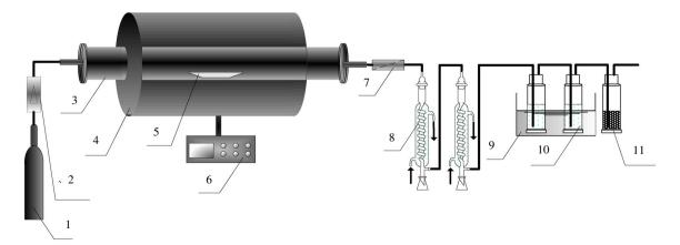
**Fig. 1** Schematic diagram of the setup of the horizontal tube furnace. *NB 1* high-pressure  $N_2$ ; 2 flow metre, 3 horizontal quartz tube, 4 quartz boat, 5 electrically heated furnace, 6 temperature controller, 7
